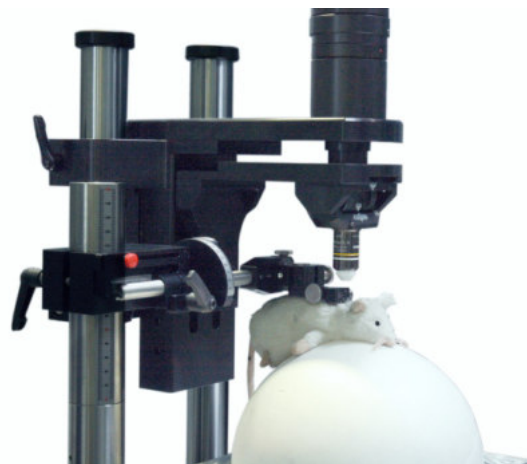
LN scope with headpostholder and virtual reality jetball
