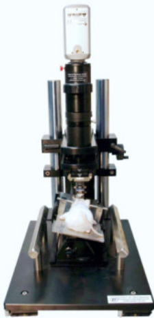
LNscope with InVivo Stereotaxic platform and InVivo angle table
